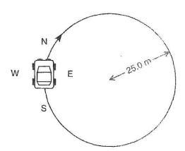
What minimum friction force must exist between the tires and the road to prevent the car from skidding as it rounds the curve?
