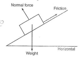
If the box is at rest, the net force acting on it is equal to
