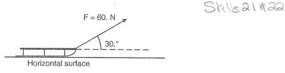
259. Determine the magnitude of the frictional force acting on the sled.
