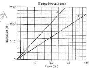
Compared to the spring constant for spring A, the spring constant for spring B is
