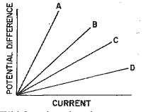
Which resistor has the greatest resistance?
