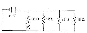
How much power is dissipated in the 36-ohm resistor? (SKill 41,44)
