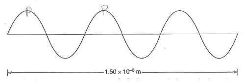
341. A periodic wave travels at speed v through medium A. The wave passes with all its energy into medium B. The speed of the wave through medium B is  $\frac{v}{2}$ . On the diagram below draw the wave as it travels through medium B. [Show at least one full wave.]
