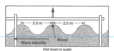
344. Calculate the speed of the water waves. [Show all work, including the equation and substitution with units.]
