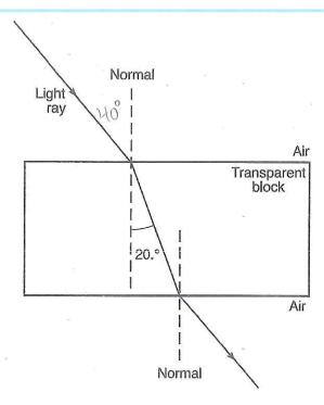
327. Calculate the absolute index of refraction for the medium of the transparent block. [Show all work, including the equation and substitution with units.]
