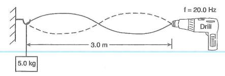
329. Calculate the speed of the wave in the rope. [Show all work, including the equation and substitution with units.]
