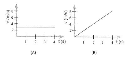
Determine the displacement for the first 3s.
