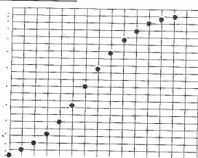
This object speeds up for 0.5 seconds, moves at constant speed for 0.2 seconds, and slows down for 0.6 seconds.
