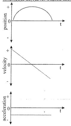
The 3 graphs at left summarize the motion of vertically launched projectile with respect to time for position (d vs t), velocity (v vs t) and acceleration. For objects launched upward, the reference point is the ground:
