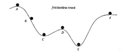
In the track above the total mechanical energy is always equal to the PE at A or the KE at E (assume that is ground level). The energy is redistributed as KE and PE depending on changes in height.
