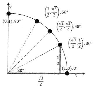
In order to use this chart to estimate resultants based on known components or vice versa, remember to follow the format of "x" and then "y" where the angle  $\Theta$  is measured between the horizontal component and the resultant.
