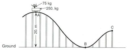
104. Compare the total mechanical energy of the car and passenger at points A, B, and C.
