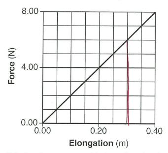
Calculate the energy stored in the spring when the elongation is 0.30 meter. [Show all work, including the equation and substitution with units.]
