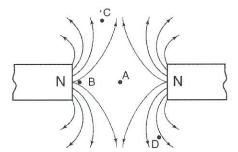
At which point is the magnetic field strength greatest?
