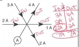
What is the reading of ammeter A?
