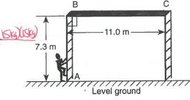
What is the angle of the painter's displacement relative to the horizontal as they move from A to C?
